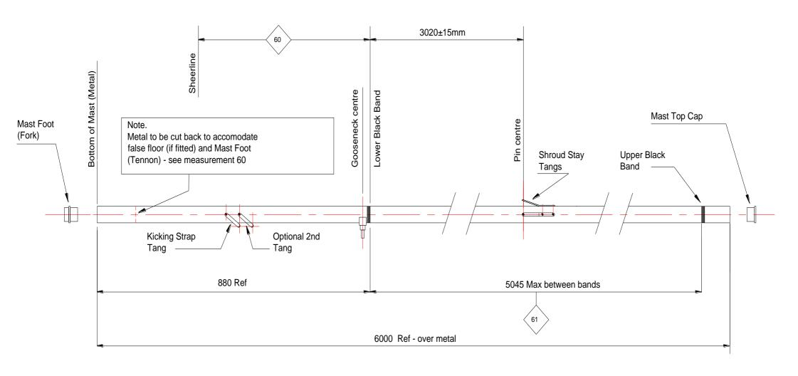
STREAKER ALLOY MAST - Supplied by :-Selden - LAMBDA Section or Superspars - MHR Section
