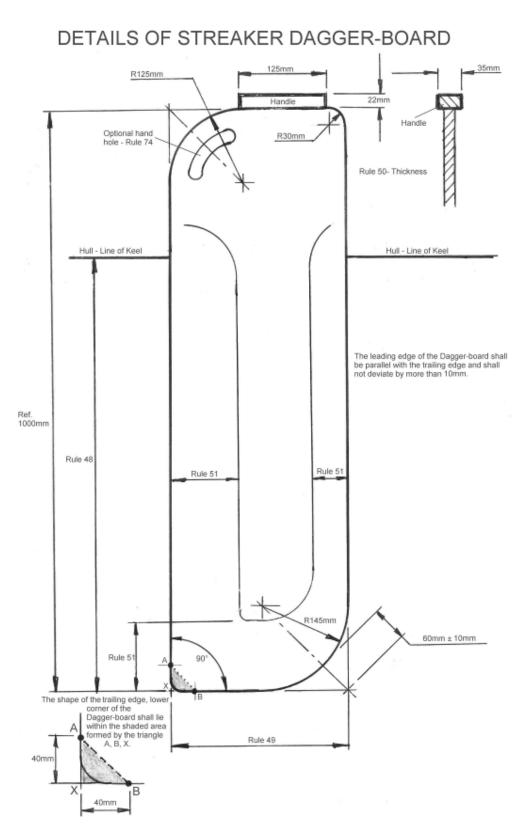
It should be noted that the Dagger-board is fitted with a handle. Whilst the handle as shown is as per the size and shape from the list of parts as supplied with the original wood kit, the important detail is that a handle is fitted. The handle acts as a positive stop which limits the depth of the Dagger-board below the hull. Pieces of rope tied through holes drilled through the dagger-board are not acceptable as a stop.
