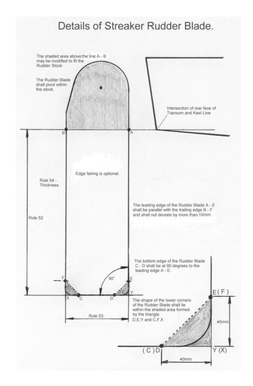
In the Rudder Blade the corners can be square or any other shape as long as the corner profile is fully contained inside the 40mm right-angle triangle.
