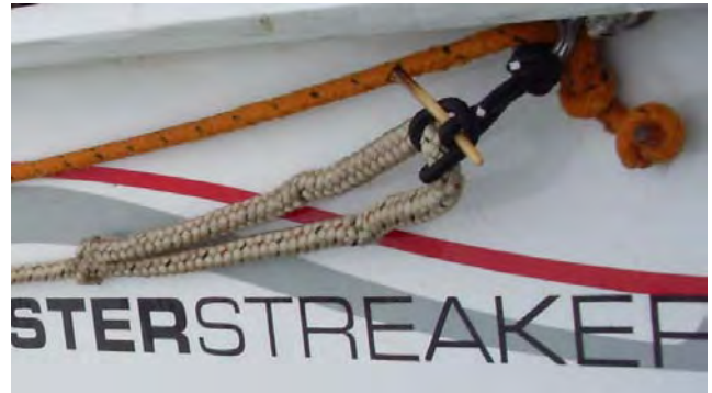
Aft fastening with quick-release mechanism, under mainsheet traveller deck eye
