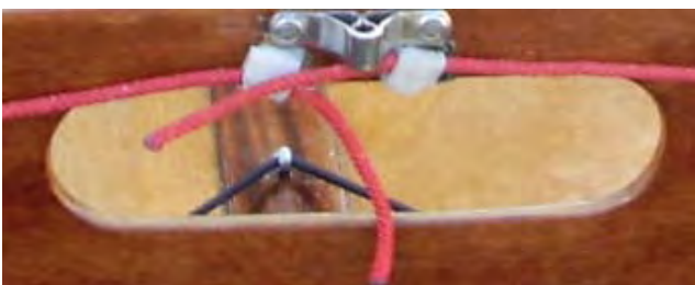
Righting lines secured at the transom with Velcro (on a Solo)
