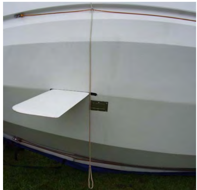
Righting line correctly positioned, behind dagger board
