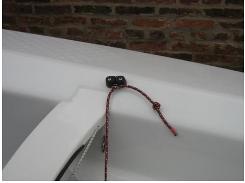
My kicker allows me to pull it on until the control line comes over my shoulder and it is where I can get at it whilst sitting out on both sides of the boat.
