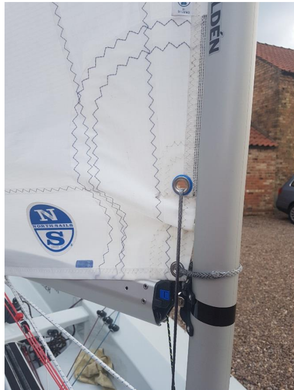
Downhaul on (Note how far the cunningham hole has been pulled down below the word Selden on the mast.)
