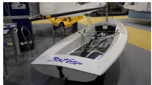
As can be seen, the boat sported a Super Spars carbon boom and a centre-mainsheet with track and traveller.
