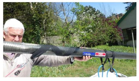
Using a webbing strap, held back to a point further down the boom, is commonly used in other classes (e.g. the Phantom, as in the photo) and means you don't have to drill holes for attaching fittings where the pull of the kicker is strongest. Now, as Alan has explained, we can do this too with dispensation.
